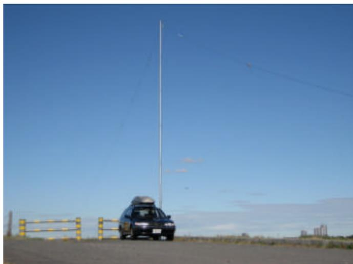
Dipole antenna 3.5MHz-28MHz
