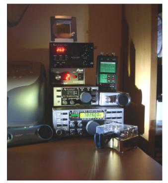
The picture shows my QRP rigs which were all homebrewed by me. We can see K2, K1, SST, T1 a tiny auto-tuner and KX1. I have many rigs enough for QRV, but I am lack of good antenna. So I use only a dipole. The Begalli Simplex Gold is pretty well for CW operation, and I love operating with this paddle at my ham shcak. To QRV with these homebrewed rigs is also one of the aims of this year.
