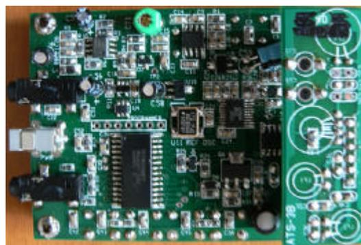
It is small transceiver kit designed and sold by Steven, KD1JV. "The ATS series started out as a SMT project in an attempt to build a trail friendly rig into an Altoids tin.", he posted to the AT\_Sprint reflector. It has a DDS VFO and can be on 80-meter through 15-meter by replacing the plug-in filter boards.
