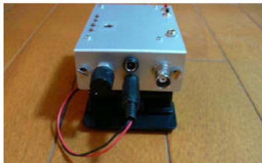
My ATS-3B can put out about 1 watt @ 6 volts, and 5 watts @ 12 volts. I set it into the enclosure, which is larger a little bit, and added some parts to operate comfortably.
