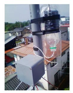
Two years ago Elecraft K1 was added to my rig collection. Soon later I got a K2 and constructed it. Since then it has been my main rig for HF bands. Last year I built up a 40m band GP for HF on the roof of the house, using a fishing rod and a small loading coil winded around a PET bottle.
