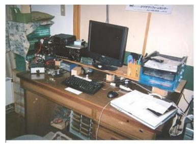
At the left side on the desk there are Bencher K-3, a memory keyer, and Bencher JA-2, a keyboard. A white case at right side of the desk is a spare laptop PC. The photo doesn't show the main laptop PC.
