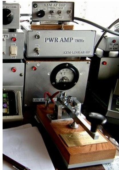
Closeup of 10 W power amplifier and a key "Takumi" manufactured by GHD key.
