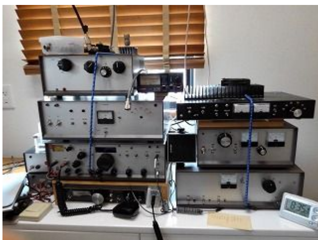
My solid-state transceiver, transverters and linear amplifier for 3.5, 7, 14, 18 and 21MHz CW/SSB.
