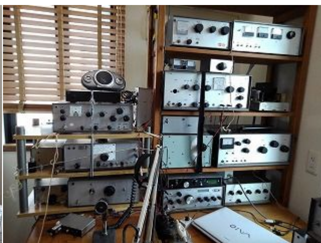
My tube type transmitters, amplifiers, crystal converter and solid-state receiver. Mainly used for 7MHz CW and SSB.
