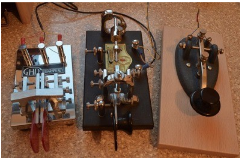
GHD paddles, 30 year old Vibroplex original and "Wilson" straight key that I've used for 60 years. The Wilson key is a fairly common Canadian key dating from WWII.
