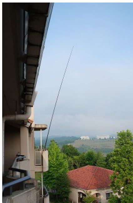
JO3HPM. The nine metre wire along the fibre grass pole on a balcony enable me to QRV from 80 m to 10 m.
