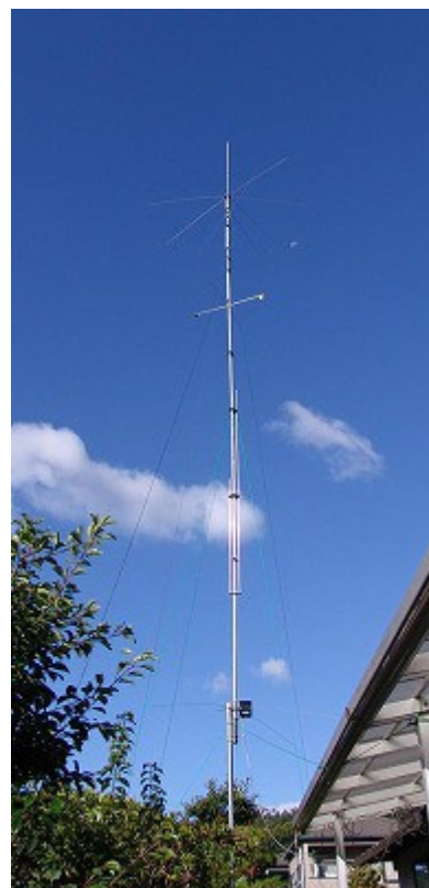
Fig. 1 Cushcraft R9 installed in my garden (you can see a half moon near the top radials)
