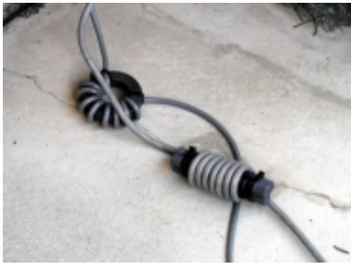
Picture 3: ICOM AH-4's cables at the entry point of my room, with a 3D-2V coax of 10 turns wound on an FT-240-61, and a control cable of 7 turns wound on a triangular stick of 3 ferrite bars. The distance between the entry point and the AH-4 is about 4 to 5 meters, which consists of the height of the balcony wall and the ground. This length is quite adequate to resonate HF high band frequencies, so I have added another pieces of cores as shown in Picture 3 at the outdoor-side of the entry point.
