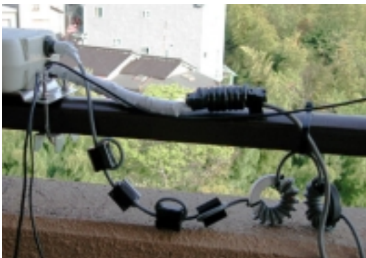
Picture 2: ICOM AH-4, with a control cable of 10 clamp cores shielded by white vinyl tape and wound on a thick triangular stick of 3 ferrite bars, and a 3D-2V (almost equivalent to RG-58/u) feeding coax with 4clamp cores, 10 turns wound on an FT-240-43 troidal core, and another 10 turns wound on an FT-240-61 troidal core.
