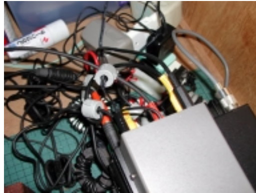
Picture 5: Almost all outputs and inputs of IC-706mkIIIG, SCAF-1, and DM-330MV are protected by a common-mode filter of clamp cores, toroidal cores, or ferrite bars.
