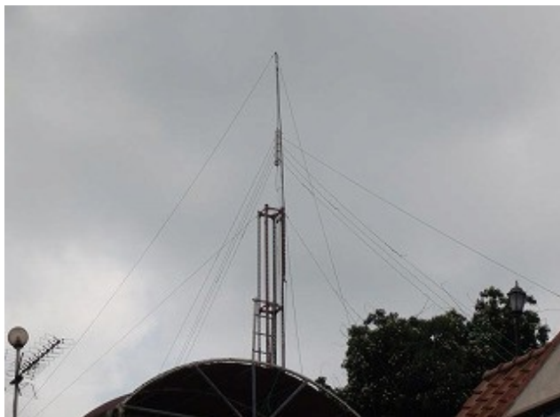
My Current Antenna: Inverted V Fan Dipole Tuning 40, 20, 15, 10 and 6 metres
