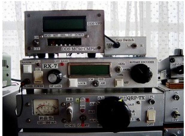
DDS-VFO: KEM-DDS-VFO-MC50 (for TX), RX: KEM-RX7-DX, TX: MIZUHO QP-7
