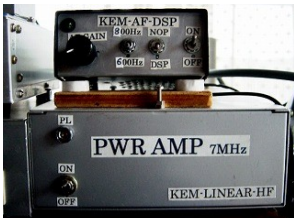
DSP: KEM-AF-DSP, 10W PWR AMP: KEM-LINEAR-HF
