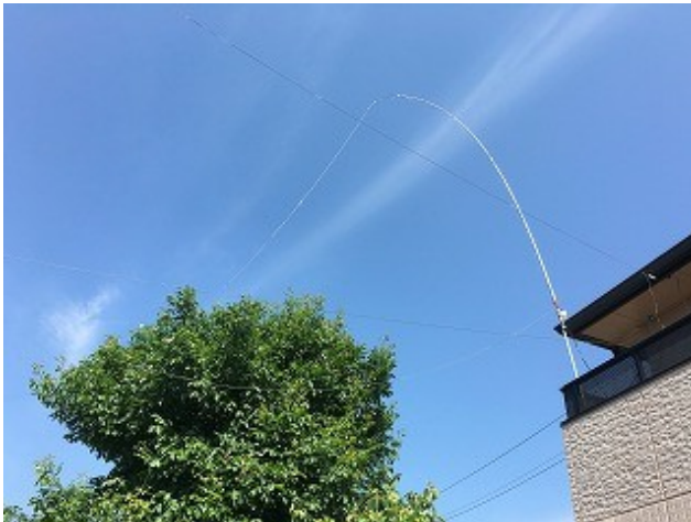
my simple antenna for 17 meter band
