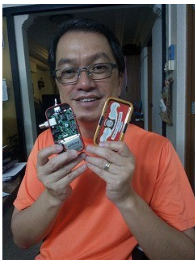
My first project: - A QRP Pixie DIY kit built and cased inside a candy box.
