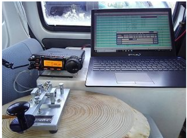
The photo shows my radio, FT857DM mounted on my car with a straight key GT503A. I enjoy pounding CQ on 7MHz CW.
