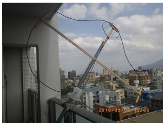
A larger magnetic loop for 7 MHz with a single main loop of a 5D2V coaxial cable.
