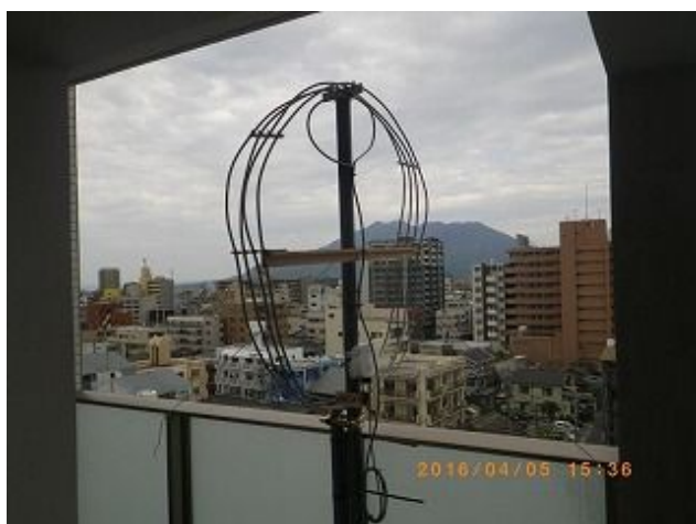
A small magnetic loop for 7 MHz using a bundle of coaxial cables (not multi-turn).
